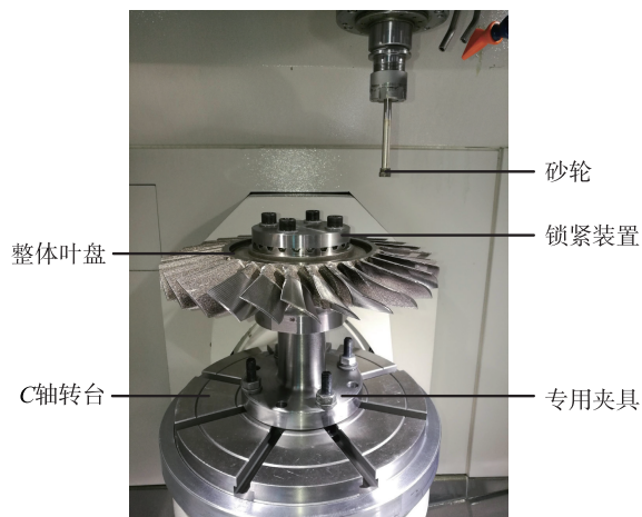
图13 整体叶盘安装图 Fig.13 Diagram of blisk installation
